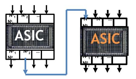
Connection between two chips is composition of two first order functions
